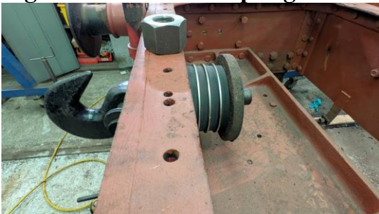
Fig 16. Reworked coupling hook being trial fitted.
