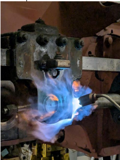
Fig 27. The crosshead here is being heated to expand it while force was being applied to the piston rod. Note: we spotted the screw was not correctly positioned and it was rectified prior to continuing.
