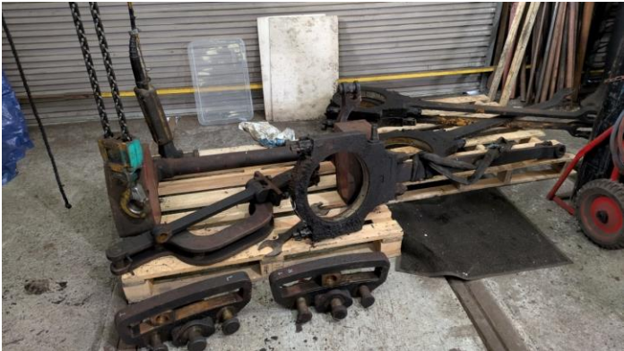
Fig 23. Valve gear parts removed, in the foreground the expansion links, the omega shaped part is an intermediate valve rod that dodges over the leading axle, and eccentric straps and rods behind.
