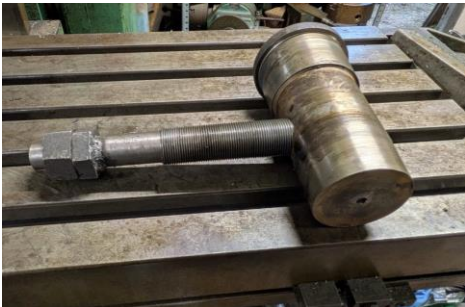
Fig 26. The dummy gudgeon pin with the fine pitched screw used to apply pressure onto the piston rod.
