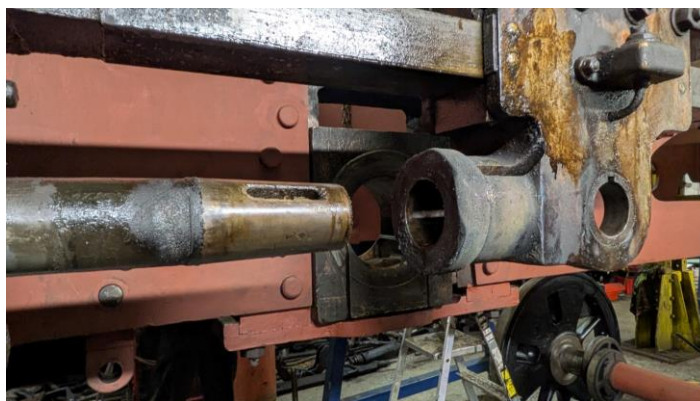
Fig 13. Here you can see the taper on the piston rod that fits into a matching one in the crosshead. Also the slots in both items that take the key that retain the parts in case of shock loadings such as water trapped in the cylinders.
