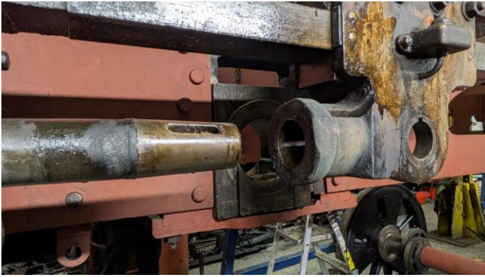
Fig 28. Here you can see the taper on the piston rod that fits into a matching one in the crosshead. Also the slots in both items that take the key that retain the parts in case of shock loadings . For example water trapped in the cylinders.
