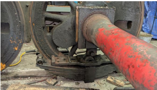
Fig 21. The horn stay on top of the spring and the axle passing through the axlebox.
