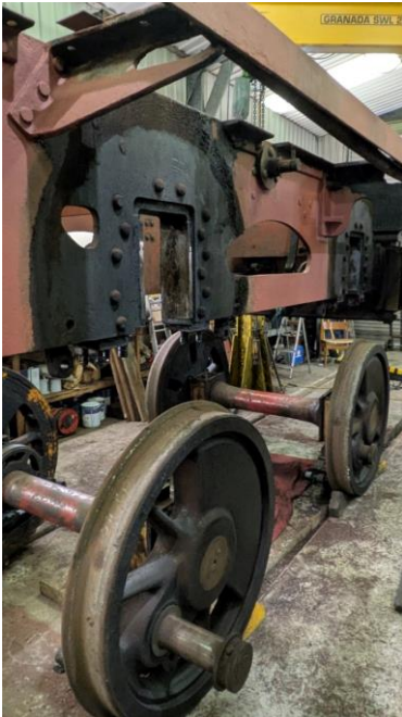
Fig 8. The frames now lifted, the wheels still on the rails. Note the dirt behind the area previously made inaccessible by the wheels.
