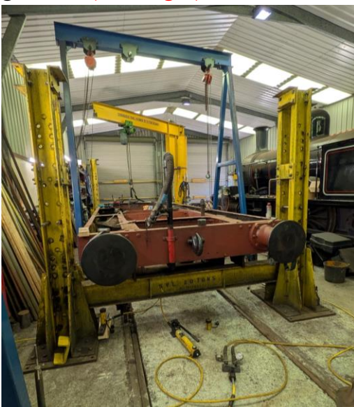
Fig 6. The lifting beams in place under the frames ready for lifting.
