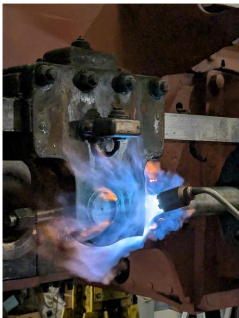
Fig 12. The crosshead here is being heated to expand It while force was being applied to the piston rod.
