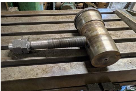
Fig 11. The dummy gudgeon pin with the fine pitched screw used to apply pressure onto the piston rod.
