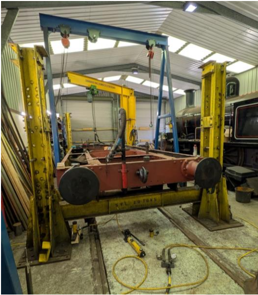
Fig 20. The lifting beams in place under the frames ready for lifting.
