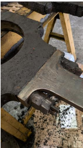
Fig 24. To the left is the dirty eccentric strap as taken off of the engine, the rod to the right has been cleaned.
