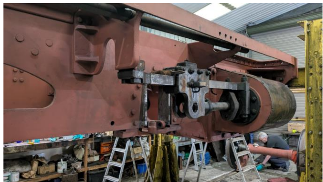
Fig 5. The frames now cleaned, needle gunned and in primer.
