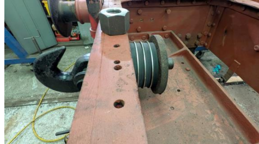
Fig 2. Reworked coupling hook being trial fitted New nut can be seen on top of the framing
