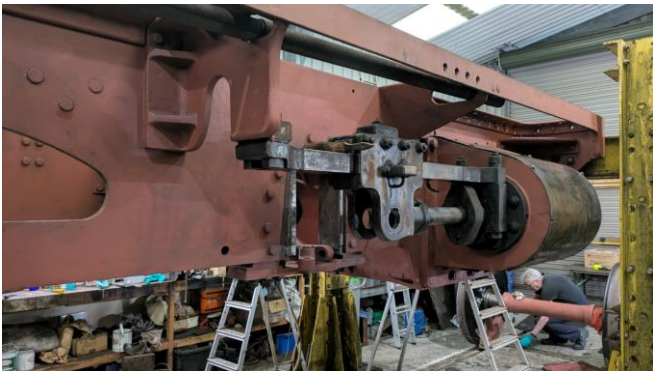
Fig 19. The frames now cleaned, needle gunned and in primer.
