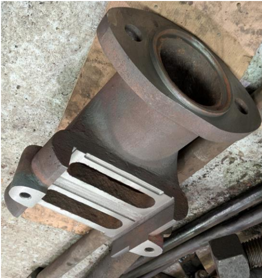
Fig 29. Here is the re-machined regulator body. When will this be installed!
