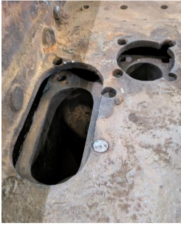
Fig 17. the plate over laying the valve chests. The cut off stud near the front shows the problem. Bear in mind these studs are firmly rusted into their threaded holes.
