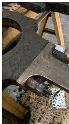
Fig 10 To the left is the dirty eccentric strap as removed and, on the right, the cleaned version.
