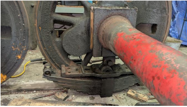
Fig 7. The horn stay on top of the spring and the axle passing through the axlebox.
